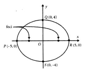
The foci are at (-3, 0) and (3, 0).  $\overline{PR}$  is the **major axis**, and  $\overline{QS}$  is the **minor axis**. This ellipse is symmetrical about both the *x*- and *y*-axes.
