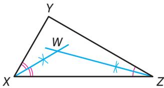
Draw a triangle  $XYZ$  and construct two angle bisectors of the triangle to locate the incenter  $W$ .
