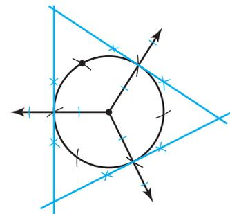
Construct a line perpendicular to each of the rays.
