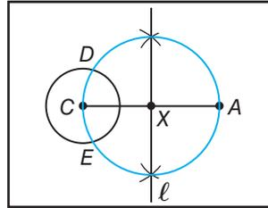
**Step 4** Draw  $\overleftrightarrow{AD}$  and  $\overline{DC}$ .  $\triangle ADC$  is inscribed in a semicircle. So,  $\angle ADC$  is a right angle and  $\overleftrightarrow{AD}$  is tangent to  $\odot C$ .
