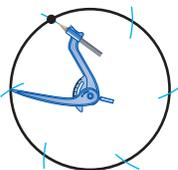
Construct a circle and draw a point. Use the same compass setting you used to construct the circle to construct an arc on the circle from the point. Continue as shown.
